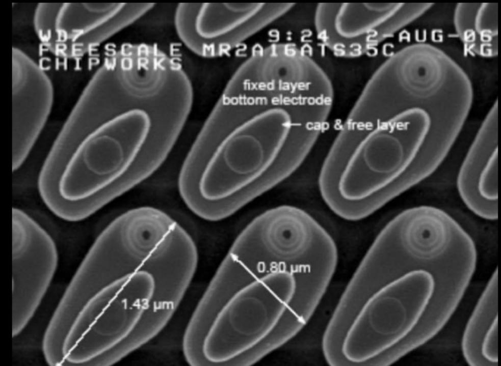
Magnetic Tunnel Junction Top View
