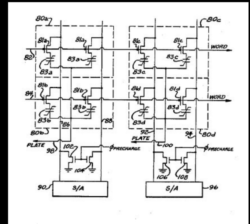
Ramtron Patented 1T-1C FRAM Cell
