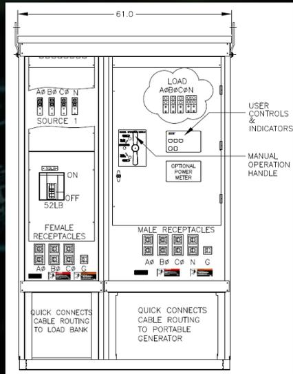
**MTDQ – Dual Purpose Manual Transfer Switch with Quick Connects**
